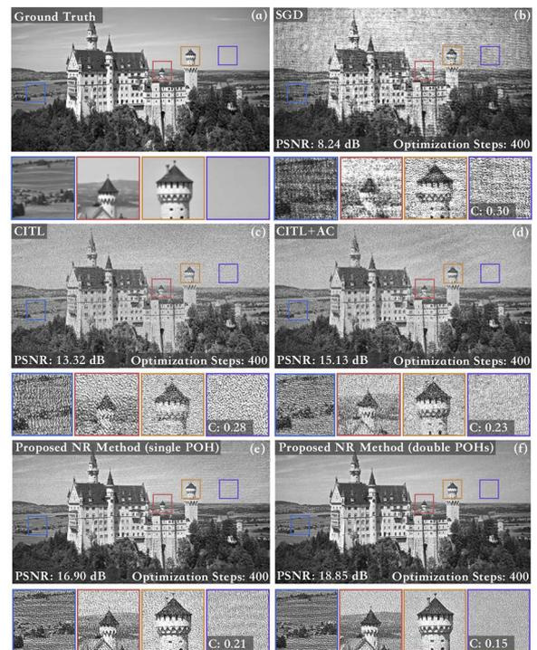
**Fig. 5.** Experimental results. (a) Ground truth image. Results of the (b) SGD, (c) CITL, (d) CITL with AC, (e) the proposed NR method with single POH, and (f) the proposed NR method with double POHs.
