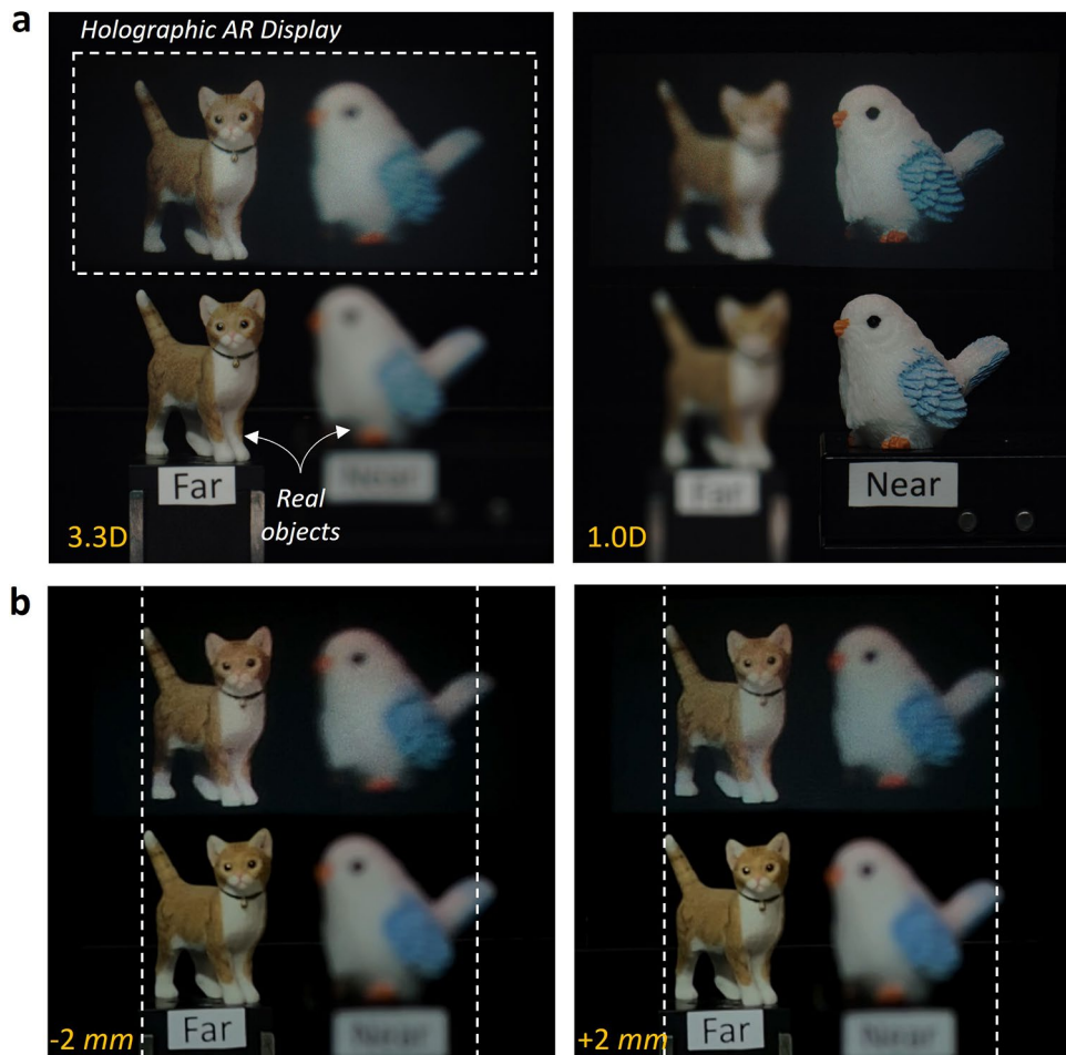
Figure 5. AR demonstration of true 3D holography featuring realistic focus cues and parallax. The real objects are placed on the 3.3D (bird) and 1.0D (cat). (a) Focal sweep results of our AR prototype, where the hologram shows realistic focus cues that of the real object. (b) Parallax results by laterally shifting the camera. Bottom insets are the shifted distance of the camera, and dot lines indicate the identical FOV in both results. The hologram and real objects are captured simultaneously.
