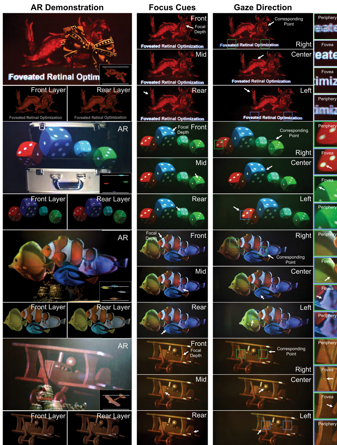
FIGURE 7. Photographs of the prototype for see-through HMD with focus cues. The first images (Chinese dragon) are display results of the system 1 with the 1.0D gap where we can observe clear pupil swim effect and focal blur. The other three images (dice, tropical fish, and toy plane) are display results of the system 2 with the 0.6D gap that can provide continuous focus cues. The see-through property is demonstrated with example applications of AR (real objects: a ribbon, box, and toys for fishbowl). Target 3D objects, layer images, focus cues, and significance of FRO are illustrated with the enlargements of the results. Gains of some enlarged images are slightly adjusted to mitigate difference in brightness for fair comparison. Additional experiment, simulation results, and sources of the 3D contents are presented in Supplementary Material.
